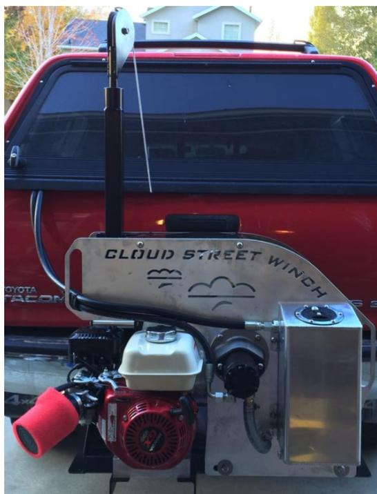
Heavy duty hydraulic payout winch with a VERY fast rewind
