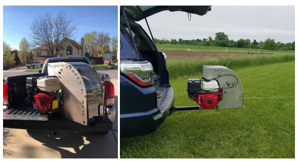
Heavy duty stationary winch Honda 390cc w/ 4' long remote throttle with kill and start switch 2500' custom woven spectra towline (2000' white, 500' red at bottom) Drogue parachute Frame is zinc base primed w/powder coat finish Trailer hitch mountable 2" x 2" Approximate weight: 185lb/84kg
