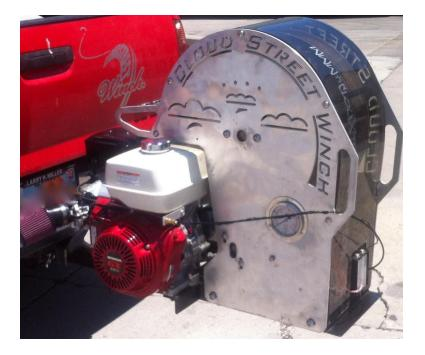
Heavy duty stationary winch with line tension guage Honda 390cc w/ 4' long remote throttle with kill and start switch 3000' custom woven spectra towline (2500' white, 500' red at bottom) Vented drogue parachute Frame is zinc base primed w/powder coat finish Trailer hitch mountable 2" x 2" Approximate weight: 250lb/113kg
